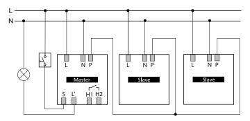
Master: thePrema S360 -101 E, thePrema P360 -101 E Slave: thePrema P360 Slave E, thePrema S360 Slave E
