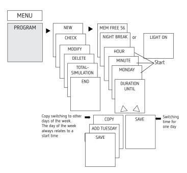
(1) A switching time always consists of a start time and an end time (LASTS UNTIL). e.g. night switch-off on Monday 23:00 - 05:00 hrs
