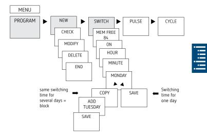
${\rm \textcircled{O}}$  A switching time always consists of a start time and an end time
