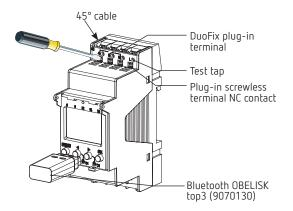
$m{\Lambda}$  Check the depth of the control cabinet when <code>OBELISK</code> top3 is connected. The depth must be > 94 mm.
