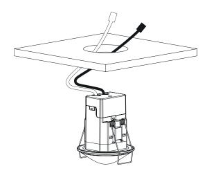
Installation in false ceilings for ceiling thicknesses of 0.5 mm to 3 cm. The diameter of ceiling cutouts must be between 62 mm and 70 mm.
