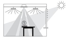
Room correction factor = Brightness value at the ceiling / brightness value at the working surface
