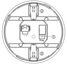
① Programming mode button② Mechanical safety lock
