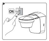
> Connect motion detector to power supply.
