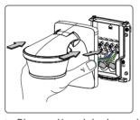
➤ Plug motion detector onto base and engage.
