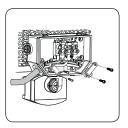
➤ Fix cord grip and tighten screws
