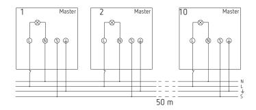
The S connection must be conducted through the same cable as the L and N line.
