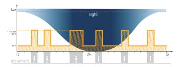
The LED spotlight shines permanently with a basic brightness of 30 %. It always switches on when there is motion (to 100 % brightness), independent of the surrounding brightness.
