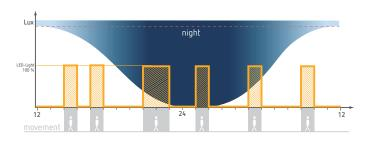
① The LED spotlight always switches on when there is motion, independent of the surrounding brightness.
