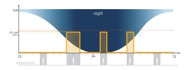
① The LED spotlight switches on when there is motion in the dark.
