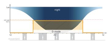
The motion detector only reacts to brightness. The LED spotlight is always switched on when the set brightness value has not been reached.
