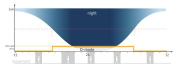
① The motion detector only reacts to brightness. The LED spotlight is always set to 30 % when the set brightness value has not been reached.
