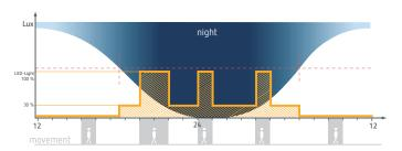
① The LED spotlight shines in darkness with the set 30 %. In case of motion, it switches to 100 %.
