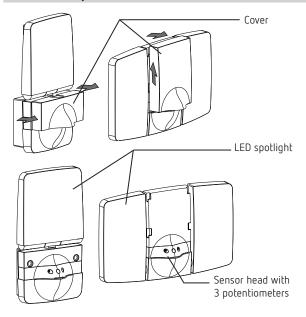
The LED spotlight has 3 potentiometers for setting time (min), brightness (lux), and function mode.
