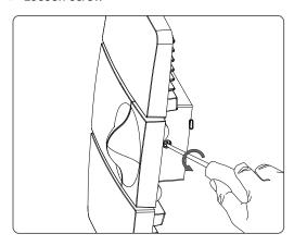
➤ Loosen catch mechanisms with a screwdriver and remove LED spotlight from base
