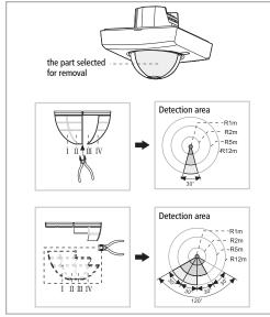
Secure cover: remove cover and attach relevant baffles:
