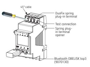
Check the depth of the control cabinet when OBELISK top3 is connected. The depth must be > 94 mm.
