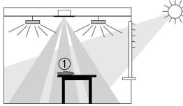
Room correction factor = Brightness value at the ceiling / brightness value at the working surface
