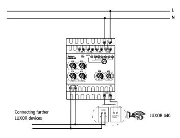
The operating voltage is extra-low voltage SELV. The COM port is function low voltage FELV.
