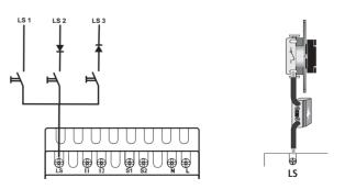
Do not connect the input of the light settings of several devices in parallel.
