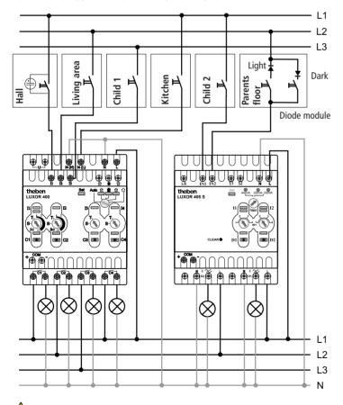
**Do not connect the inputs in parallel.**
