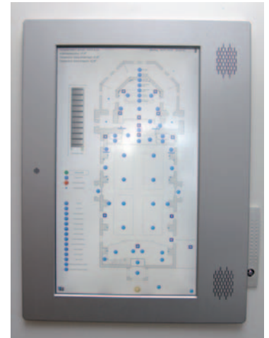
The visualisation on the 22-inch touchscreen with church layout provides clear view of lighting functions.
