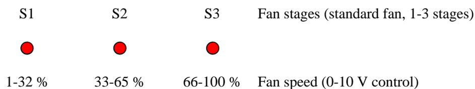
By using the manual button, the fan stages can be switched one after another.
