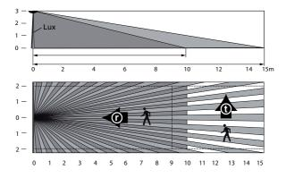
Because of the virtually horizontal detection of compact passimo, the detection range of tangential (t) movements of persons is different to the range of radial (r) movements towards the detector.
