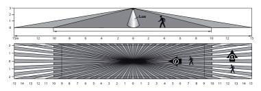
**Please note:** because of the virtually horizontal detection of compact passage to both directions, the detection range of tangential **(t)** movements of persons is different to the range of radial **(r)** movements towards the detector.
