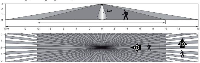
15 14 13 12 11 10 9 8 7 6 5 4 3 2 The detection range in side view (top) and top view (bottom).
