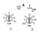
If setting values for brightness <= 2.5 AND switch-off delay time light <= 2 min: faster response to changes in actual brightness when in operating mode switching of one lighting row.
