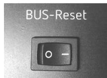
Afterwards, all parameters and programming settings for the KNX devices will have been deleted and the physical address will once again be 15.15.255.
