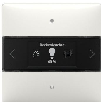
The iON 108 KNX room controller with integrated temperature sensor can be used in residential buildings, meeting rooms and offices, as well as in commercial buildings. It is mounted on a standard junction box using the supplied mounting plate. Combinations of two iON KNX are possible with a 2-way mounting plate available as an accessory. The integrated bus coupling unit makes installation and connection to the bus system quick and easy.
