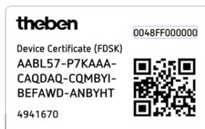
After entering the FDSK, the ETS generates a device-specific tool key. The ETS sends the tool key to the device to be configured via the bus. The transmission is encrypted and authenticated with the original and previously entered FDSK key.
