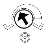
> Set the potentiometer to the desired time (5 s - 15 min.).
