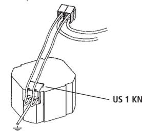
Fig. 2: Connecting the **US 1 KNX** at the existing bus terminal of the bus coupler
