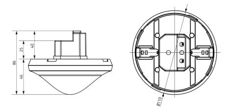
4.3.2 Surface-mounted installation and ceiling installation with springs
