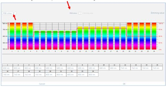
Changeover for input RGB colour – dimming value
