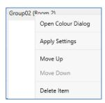
Connection to the DALI-Gateway is required. The command is performed with the value and colour settings that have been defined for this group or ECG. This makes it possible to check properties before the whole effect is programmed. If "Keep value" or "Keep colour" have been set, the respective values will not be activated, and the current value will be retained.
