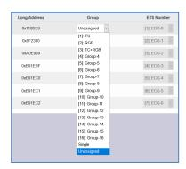
The desired assignment to the ETS ECG number can then be selected. Example: ECG with control of colour temperature with short address 1 is assigned to group 1 (TC) and ETS ECG number 2:
