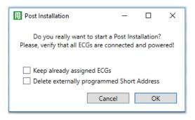
Usually, ECGs have no short address and long address 0xFFFFFF on delivery by default. It might be possible, that ECGs got a short address even if long address is still 0xFFFFFF ( i.e. if an external tool was used for programming). In order to delete short address in this case please activate the control element "Delete externally programmed short address".
