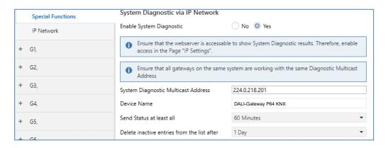
All gateways that are to communicate with each other must be configured with the same multicast address.
