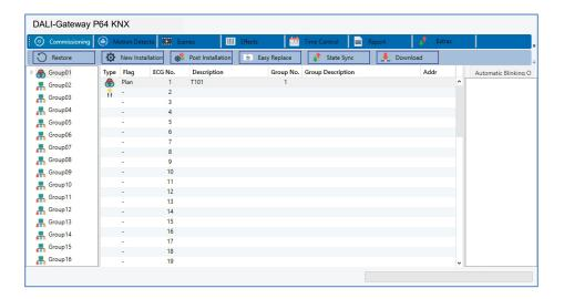
The group configuration is displayed in a tree structure on the left-hand side. The middle part shows a table for the ECG configuration and names. A list on the right-hand side shows the actual devices found in the system that have not yet been identified. During the planning phase the list is empty as the ETS is not yet connected to the system.
