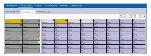
Each group is numerically and color coded and contains the respective group name. Each ECG shows the ECG number and also the respective name. In addition, the ECGs show the group memberships by a numerical and color tag. ECGs marked with an asterisk are Single ECGs. Groups and ECGs that are switched on are displayed with a yellow background.
