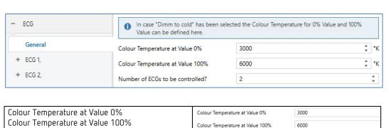
Parameters for setting the colour temperature (warm) with dimmed light and (cold) with dimmed light.
