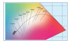
DT-8 operating devices set the required colour temperature on an LED module by mixing cool and warm white LEDs. Of course, as before this is only possible within certain physical limits. With today's LED modules colour temperatures between 2000 and 8000 Kelvin are common.
