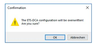
Please remember that all DCA data in the ETS will be overwritten with this data. Press the "Restore" button under commissioning in order to load the configuration onto the DALI gateway. See chapter 11.1.9 Restoring the DALI configuration.
