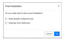
Usually, ECGs have no short address and long address 0xFFFFFF on delivery by default. It might be possible, that ECGs got a short address even if long address is still 0xFFFFFF (i.e. if an external tool was used for programming). In order to delete short address in this case please activate the control element "Reassign short address".
