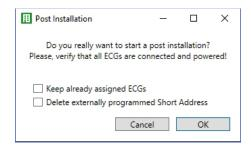
Usually, ECGs have no short address and long address 0xFFFFFF on delivery by default. It might be possible, that ECGs got a short address even if long address is still 0xFFFFFF (i.e. if an external tool was used for programming). In order to delete short address in this case please activate the control element "Delete externally programmed short address".
