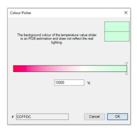
This function sets the colour temperature of DT-8 devices that support the colour temperature setting (TC). On the ECG the colour is also changed if the lamp is turned off at the time of the action. You can enter the colour temperature range. The value range permitted is between 1000 and 10000 K but please remember the physical limits of the connected ECGs and lights.
