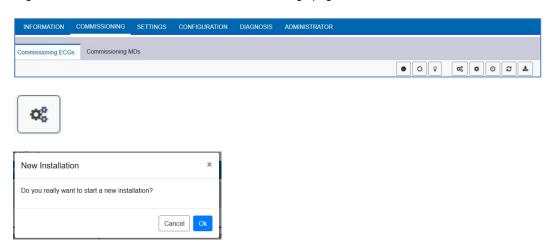
During teach-in, all ECGs are automatically detected and each ECG is assigned a short address from 0..63. The teach-in process can take up to 3 minutes, depending on the size of the connected DALI segment. The progress is shown in the popup window.
