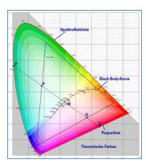
In devices that support the x-y coordinates method, the colour is set via two values between 0.0 and 1.0. However, because of the physical properties of an LED, even in an RGB LED module not every colour is practically possible. In practice, it is common to set the value which is closest.
