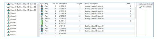
Once an ECG has been dragged into the ECG configuration table, it disappears from the list of non-identified ECGs. At the same time the 'PLAN' flag in the configuration table shows that the ECG has been assigned to the planned element. The last column in the table shows the real ECG short address.
