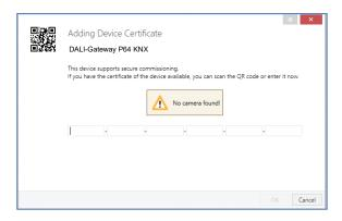
The certificate consists of the serial number and an initial key FDSK (Factory Default Setup Key). This code is only used for initial commissioning with the ETS. During the first download this key is replaced by the ETS. This prevents unauthorized persons from gaining access to the installation despite knowing the initial key.
