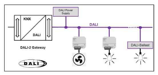
The SU 1 DALI-2 switch actuators can be used for lamps, fans, pumps, HVAC control, etc.
