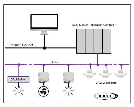
The SU 1 DALI-2 switch actuators can be used for lamps, fans, pumps, HVAC control, etc.
