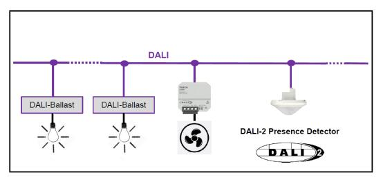
The switch actuator SU 1 DALI-2 can be used for HVAC control, etc.
