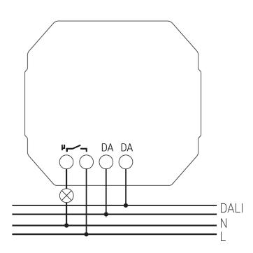
In order to ensure that the load current does not exceed the maximum permissible current of the relay, the installation must be fused with a type B or C circuit breaker of max. 13 A.
