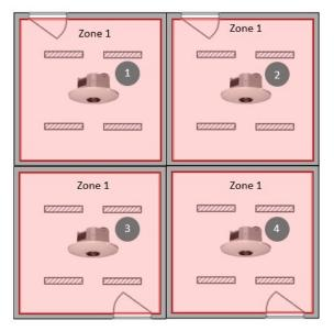
The occupancy density is evaluated in each meeting room. The detectors send the ppm value with a 16-bit output object (object 39 for zone 1), according to the respective utilisation. This ppm value can be used for an individual visualisation.
