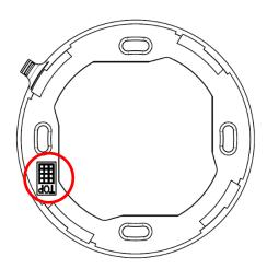
The designation TOP indicates the orientation of the detection area. Also, the area marked with TOP is displayed at the top of the screen on smartphone / tablet.
