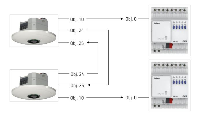
Instead of 2 different detectors, a Master-Master parallel switching can also be implemented with just one thePixa, by configuring both zones as Master.
