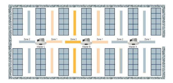
Each detector has zone 1 and zone 2 activated. Trigger objects are available for sending and receiving the motion status:
