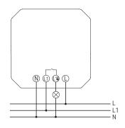
△ Secure device with an upstream type B or type C circuit breaker (EN 60898-1) with a maximum of 10.
