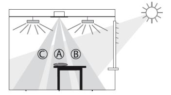
The light guide is designed in such a way that the light measurement covers an opening angle of approx.  $\pm$  40° below theRonda P360 DALI-2 S and to the side.
