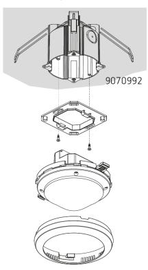
For easier installation of theRonda P360 DALI-2 S in false ceilings with thicknesses between 0.5 mm and 3 cm, a ceiling flush-mounting box 68A is available (see accessories). This also ensures cord grip and contact protection. The installation diameter is 72 mm (drill diameter 73 mm).
