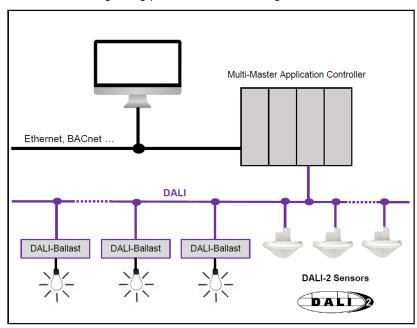
The theRonda P360 DALI-2 S presence sensor and other DALI components are connected to the DALI line. The DALI supply is provided by the higher-level system. The assignment of the short addresses and the selection of the required instances for theRonda 360 DALI-2 S are carried out via the multi-master application controller.
