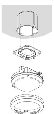
The theRonda P360 DALI-2 S is flush-mounted using a size 1 standard flush-mounting installation socket.
