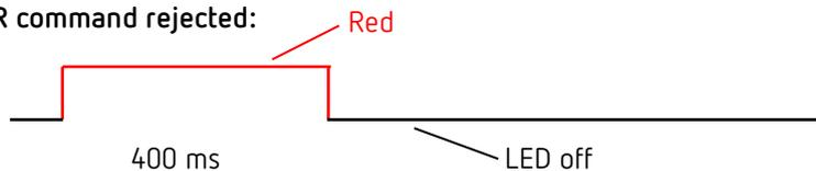
Rejection pulse when an invalid remote control command is received.
