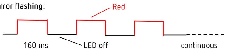
Error flashing (applies until the error has been resolved).
