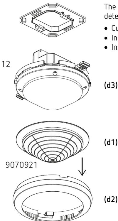
The cover clip accessory can be used to individually restrict the detection area.
