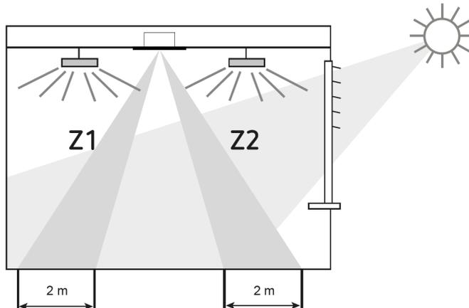
The thePassa P360 DALI-2 S presence sensor measures by means of two directed light measurements. Light measurement Z1 measures the brightness in zone 1. In zone 2, light measurement Z2 measures the brightness. Each light measurement zone maps a rectangle of about 2 x 4 m on the floor.
