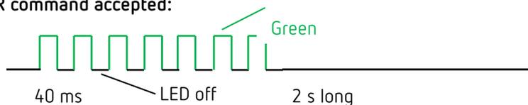
LED flickers (12.5 Hz) when a valid remote control command is received.
