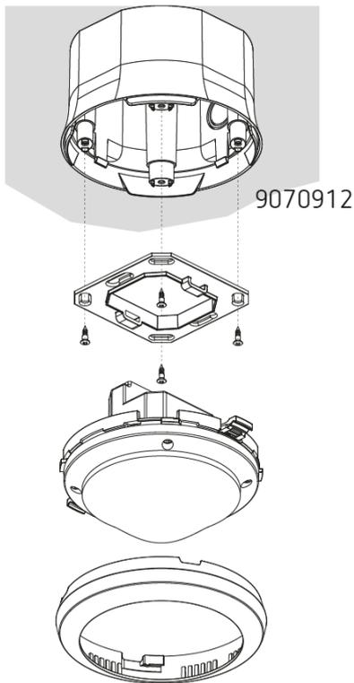
A surface frame 110A is available for surface mounted installation (see accessories).
