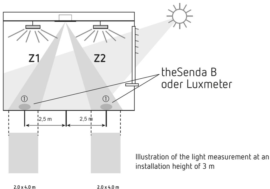
$$\text{Room correction factor} = \frac{\text{Brightness value on the ceiling}}{\text{Brightness value on the work surface}}$$
