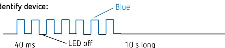
Identification of the sensor by means of the DALI command "IDENTIFY DEVICE"
