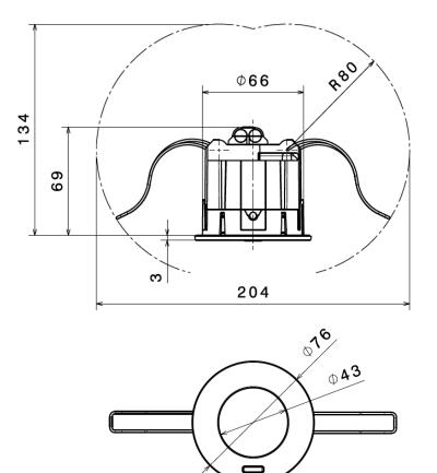
4.3.2 Surface-mounted installation with 75B back box
