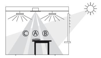
The light guide is designed in such a way that the light measurement covers an opening angle of approx.  $\pm 40^{\circ}$  below the PlanoSpot 360 DALI-2 S and to the side.
