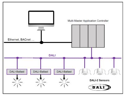
The PlanoSpot 360 DALI-2 S devices and other DALI components are connected to the DALI line. The DALI supply is provided by the higher-level system. The assignment of the short addresses and the selection of the required instances for the PlanoSpot 360 DALI-2 S devices are carried out via the multi-master application controller.
