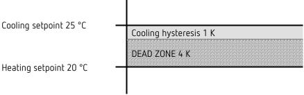
The dead zone (4 K) is increased by the value of the hysteresis (1 K) and offsets the cooling set point value to 25 °C.
