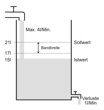
If the filling quantity is 15 I, there is a control deviation of 21 I - 15 I = 6 I As our actual value lies outside the bandwidth, the control will operate the feed at 100%, i.e. with 4 I/minute.
