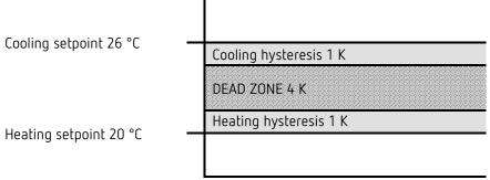
The dead zone (4 K) is increased by the value of both hysteresis (2 K) and offsets the cooling setpoint to 26  $^{\circ}$ C.
