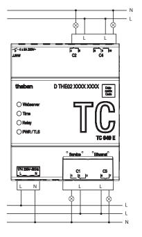
① Switch the load with a contactor.
