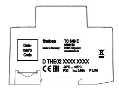
① The performance specifications can be found on the side and on the device shoulder (see picture). After installation they are not visible any more!
