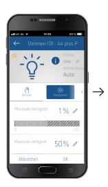
→ Functions as dimming, staircase light, comfort and settings (with alternative dimming curves) can be selected.
