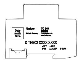
The performance specifications can be found on the side and on the device shoulder (see picture). After installation they are not visible any more!
