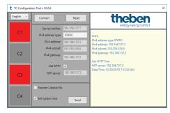
With Set system time, you can select whether the current time should be sent to the device.
