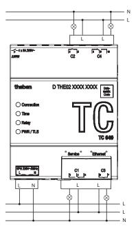
① Switch the load with a contactor.
