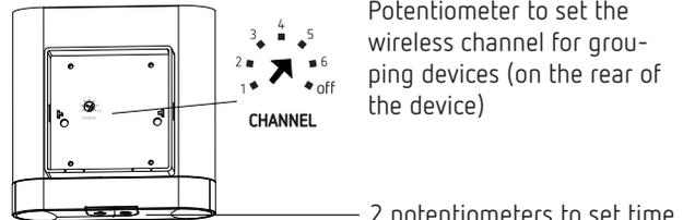
Potentiometer to set the wireless channel for grouping devices (on the rear of the device)
