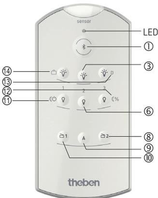
① If you would like to use the settings of the remote control for the presence detector (default) also for the outdoor detectors, press buttons 8 + 9 > 5 s.
