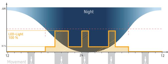
① If the brightness falls below the setpoint, the lamp switches on a reduced orientation light even without movement. When motion is detected, the light is switched to maximum brightness.
