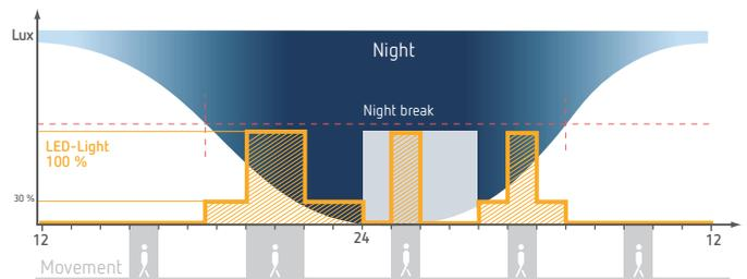
① The night switch-off does not influence the motion-triggered light switching!
