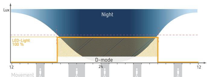
① Additional night switch-off function: switching on and off; function determines midpoint between twilight and switches off the light for 4 hours from the 2nd half of the night; function does not influence motion-triggered light switching!
