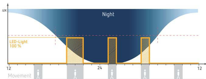
① The LED lamp is switched on if there is movement and the brightness has fallen below the setpoint.
