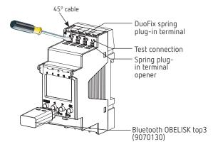
Check the depth of the control cabinet when OBELISK top3 is connected. The depth must be > 94 mm.
