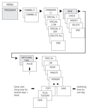
① A switching time always consists of an ON switching operation and an OFF switching operation. ① There are 84 memory cells available.
