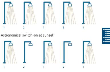
At a defined time, switch off the second channel to save energy and retain basic lighting.
