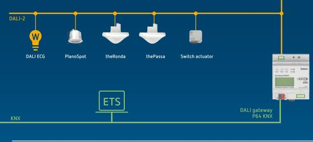
System diagram: Multi-master application controller
