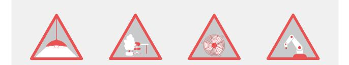
Attention: Do not install presence detectors next to suspended lamps, partitions, shelves and indoor plants or devices with moving parts such as fans, air cleaners or machines.
