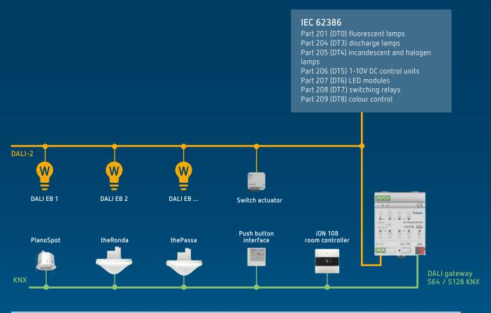
System diagram: Single-master application controller
